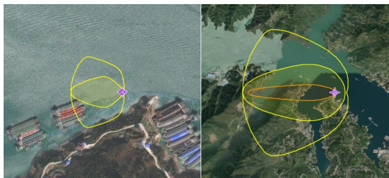
Figure 7 MARPLOT fitting results of methanol and oil and gas vapor cloud explosion areas in the waiting area
