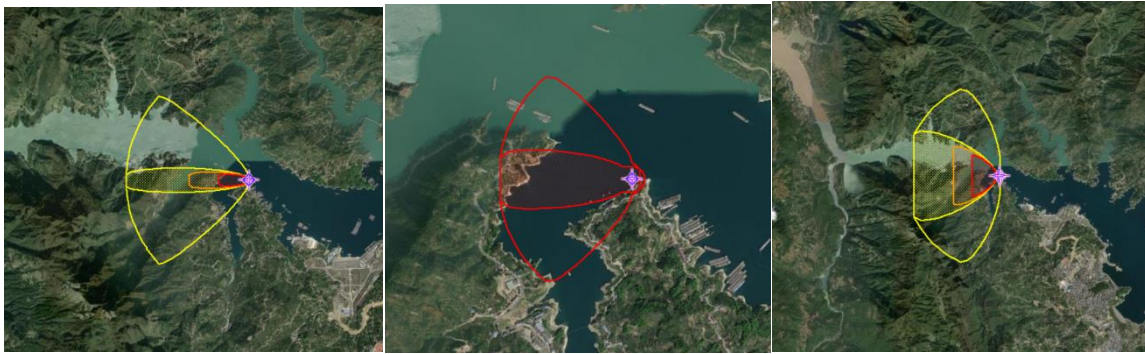
Figure 3 MARPLOT fitting results of methanol, 1, 2 xylene, oil and gas vapor cloud toxic area in the waiting area
