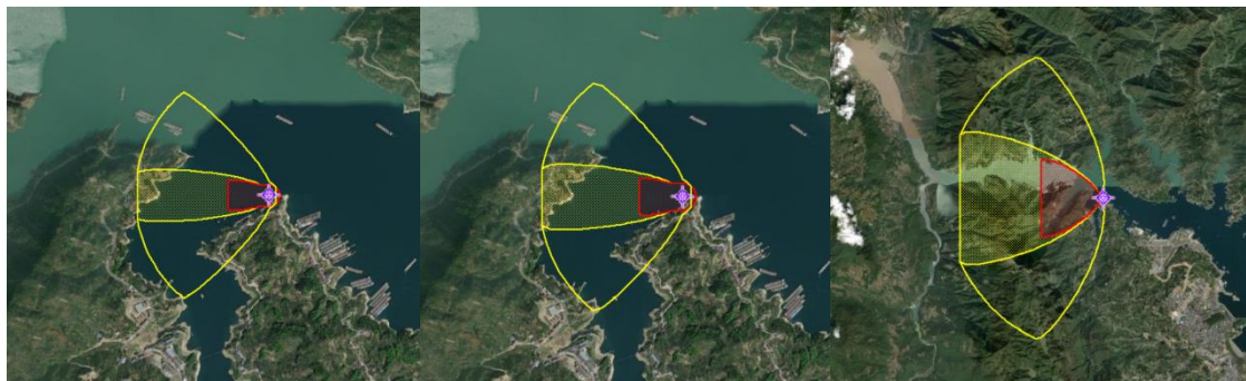
Figure 5 MARPLOT fitting results of methanol, 1, 2 xylene, oil and gas vapor cloud flammable area in the waiting area
