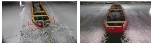
(a) The brash ice dislodged to the sides on the bow (b) The stern track of brash ice
