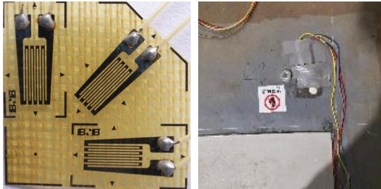
Fig.3 The resistance three-way strain rosette of BE120-3CA(11)Type
